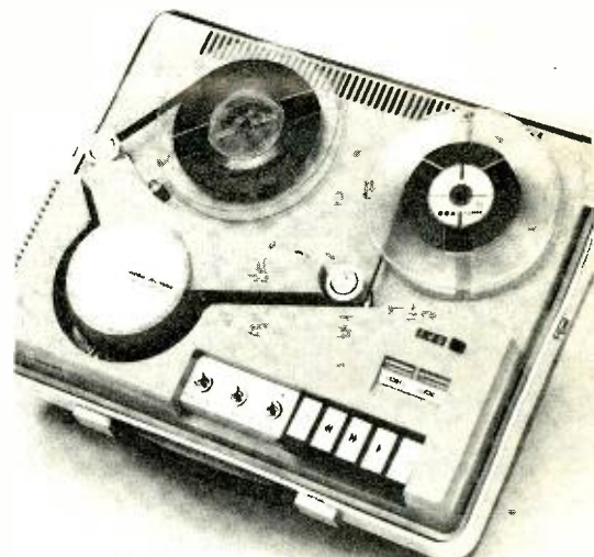
NORELCO LDL-1000 reel-to-reel video recorder/player uses 1/2-inch tape travelling at 7.9 inches/second.
