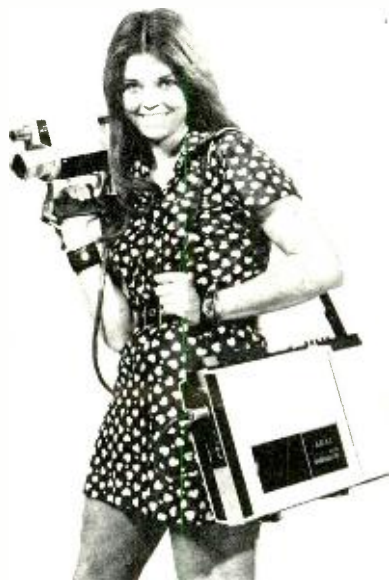
AKAI VTS-100-DX (left) uses 1/4-inch tape and includes a camera and portable 3-inch monitor.
